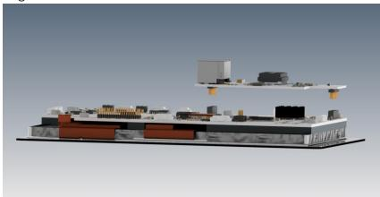
• Press the POE Add-on Board down firmly to ensure a secure connection.
