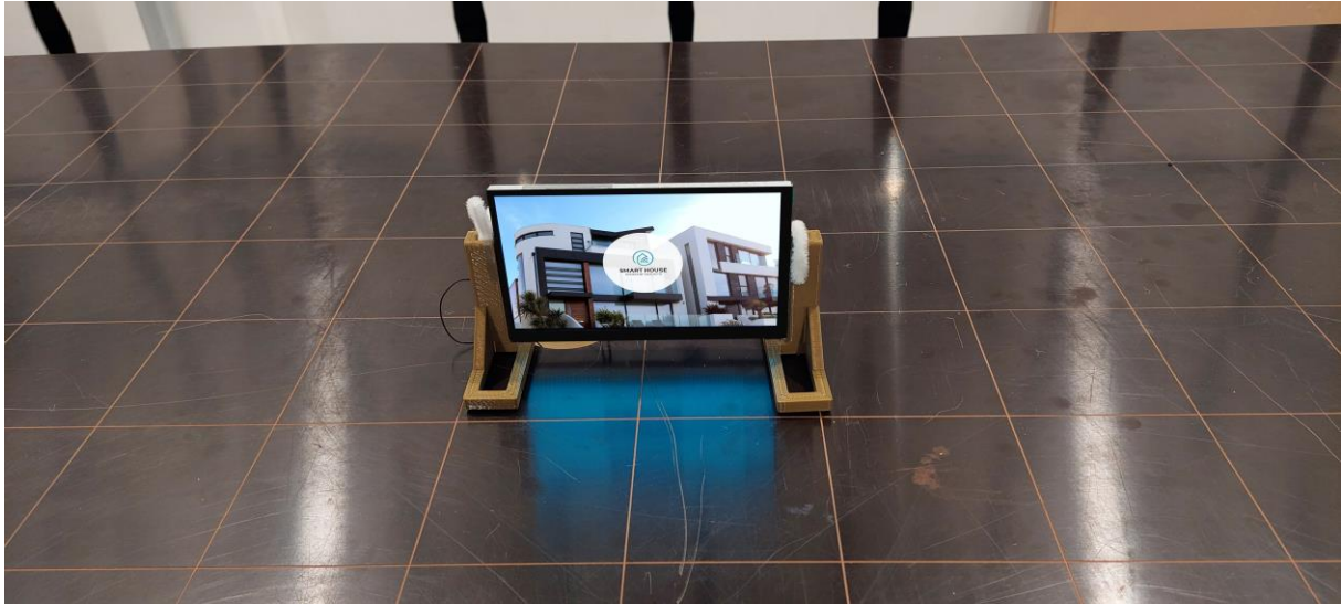
Figure 1. Radiation Emission 30-1000MHz Test Front View
