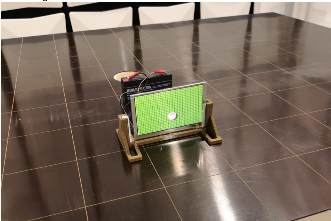
Figure 2. Radiation Emission 30-1000MHz Test Front View
