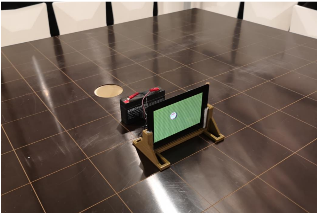
Figure 2. Radiation Emission 30-1000MHz Test Front View
