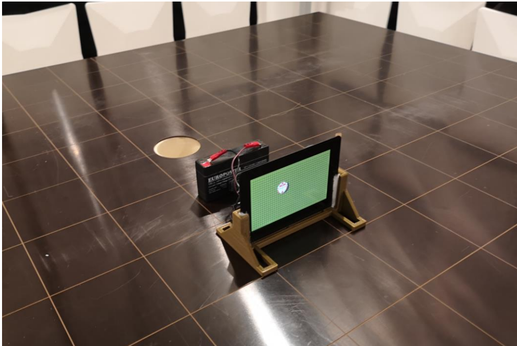
Figure 2. Radiation Emission 30-1000MHz Test Front View
