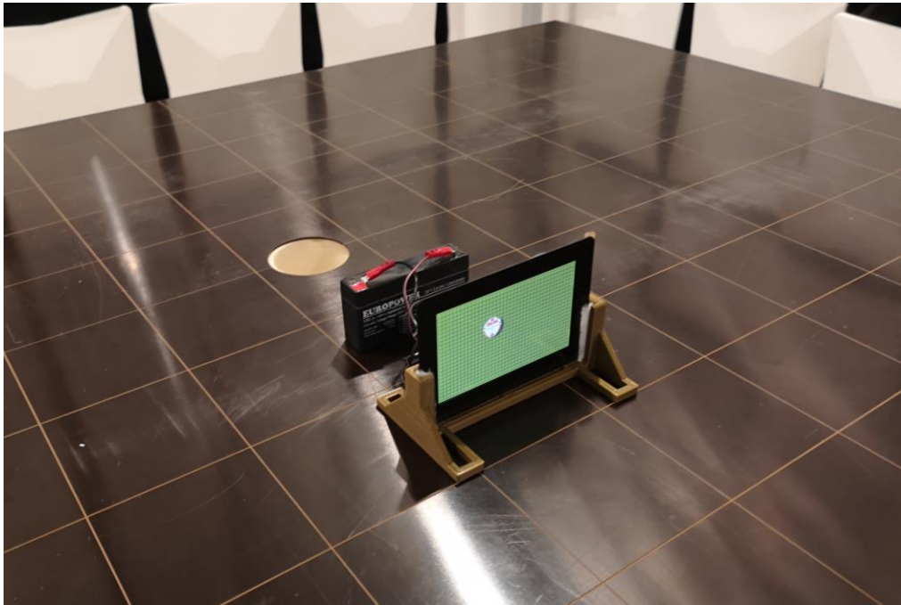
Figure 2. Radiation Emission 30-1000MHz Test Front View
