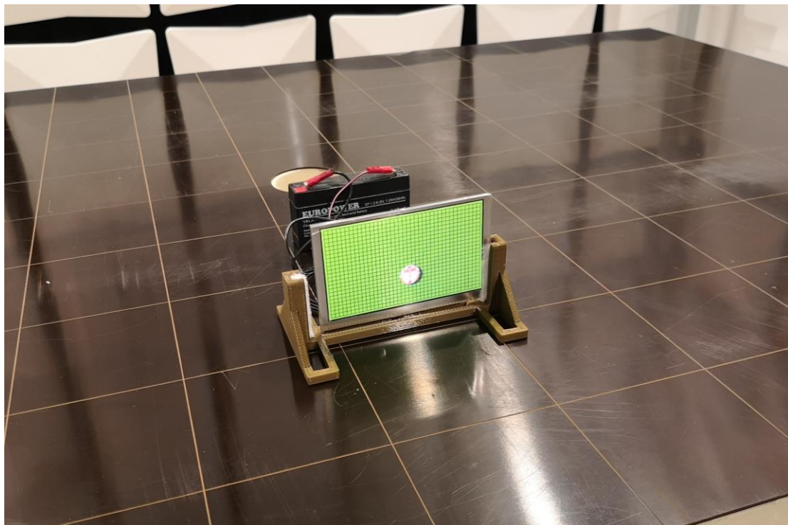
Figure 2. Radiation Emission 30-1000MHz Test Front View
