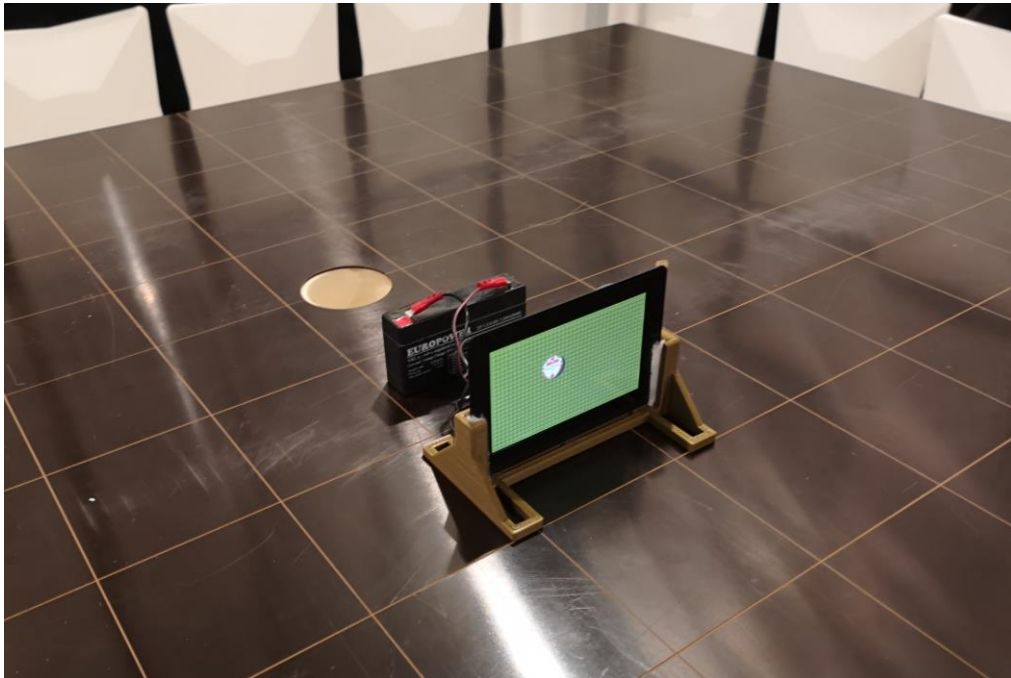
Figure 2. Radiation Emission 30-1000MHz Test Front View
