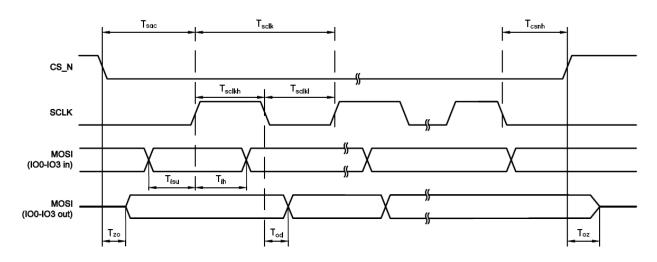
The meanings of the timings in the Figure 9 are defined in the table below.
