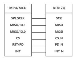
Figure 7. QSPI interface connection
