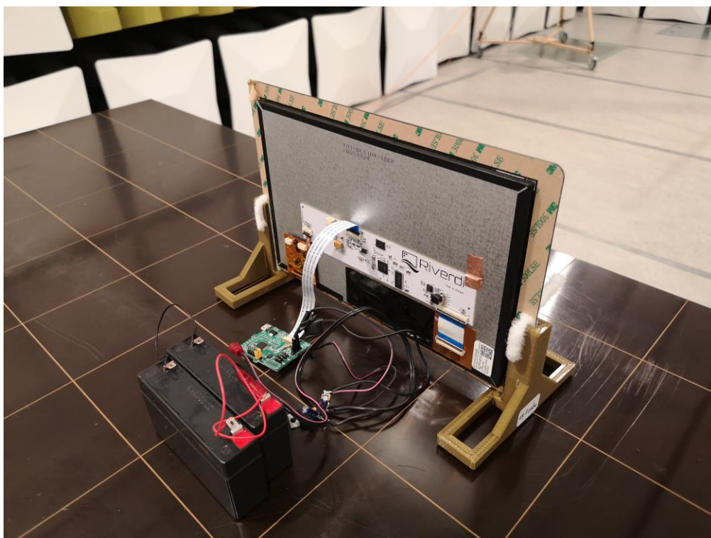
Figure 1. Radiation Emission 30-1000MHz Test Back View
