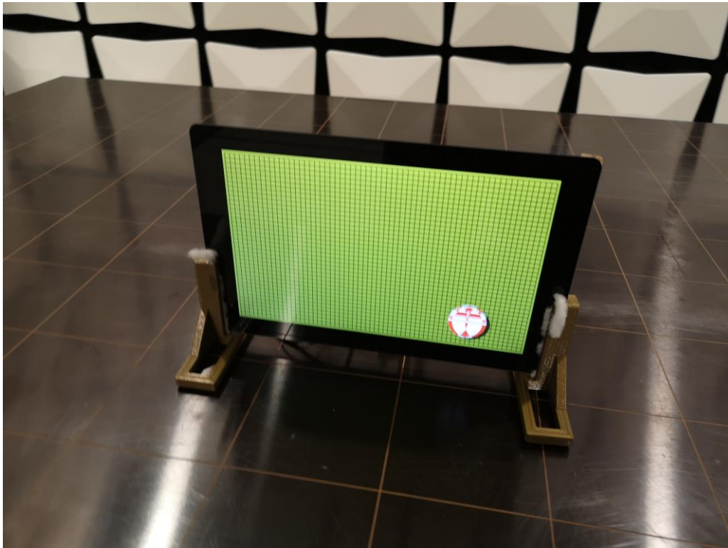
Figure 2. Radiation Emission 30-1000MHz Test Front View
