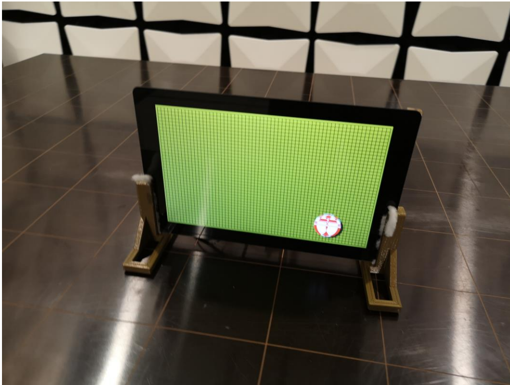
Figure 2. Radiation Emission 30-1000MHz Test Front View
