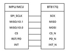
Figure 6. QSPI interface connection
