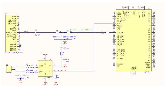
Figure 4. The simplified audio circuit design
