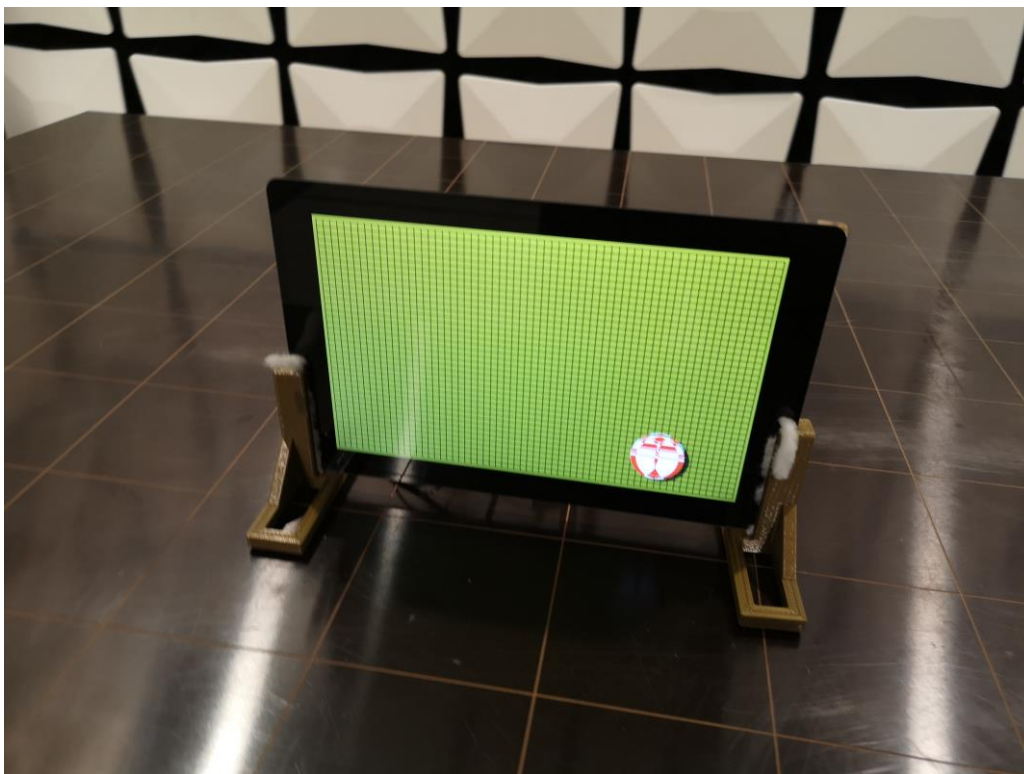
Figure 2. Radiation Emission 30-1000MHz Test Front View
