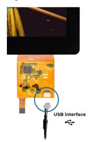
Caution! Before connecting, please make sure that the touch panel is disconnected from the touch ZIF connector on the Don Addon.
